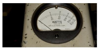
Testing of Insertion Loss/VSWR in transmit branch under actual RF power from Alinco transmitter
