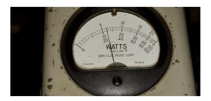
Reflected power from dummy load back to radio too low to measure, verifying proper 50 Ohm load impedance and match for reference
