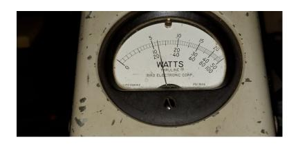
Reflected power from duplexer Tx branch back to transmitter was too low to measure, confirming excellent Return Loss, VSWR match, impedance match, and proper tuning for frequency
