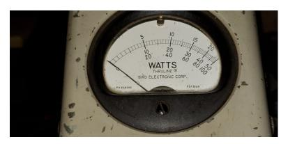
Testing with Bird wattmeter place between transmitter and input to 444.0500 MHz tuned Low Pass (Tx) Branch
