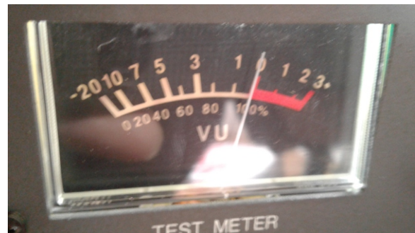
Figures 4 and 5: With front-end of receiver realigned, a -78.2 dBm signal would produce a "0" level on the Marti receiver with the receiver's 10 dB attenuation switch turned on.
