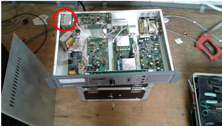
Figure 3: Marti receiver cover removed for access to tuning adjustments. The only adjustment needed was correct tuning of the three Johanson-type capacitors in the first stage filter (indicated in the circled area in the photo.)
