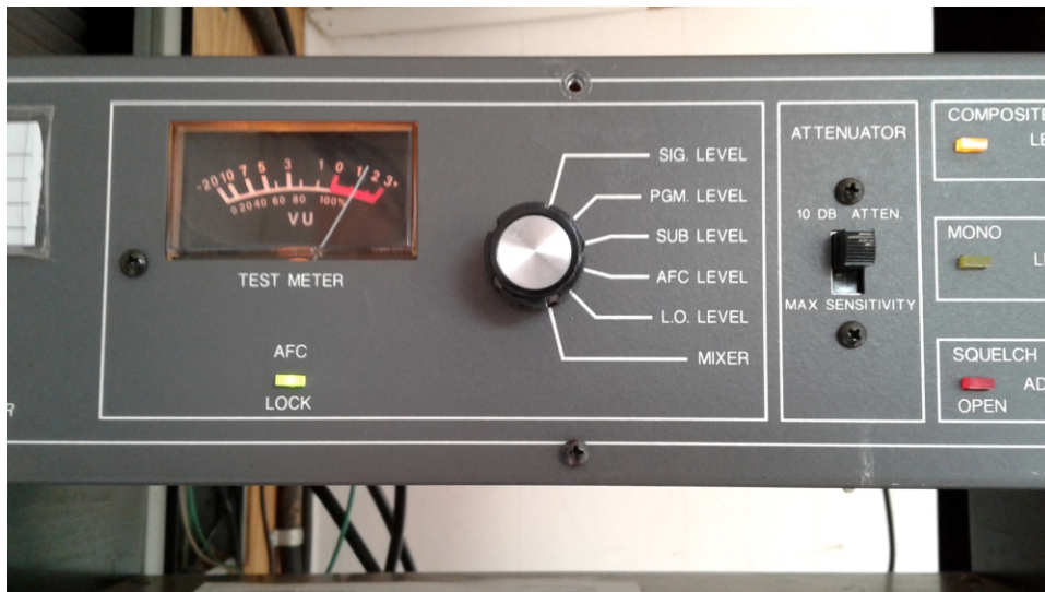
Figure 8: After STL antenna realignment, the receiver was showing just above a “+1” level on its built-in meter with the 10 dB attenuation switch turned on. I did not visit the studio to check the transmit level setting on the Marti STL transmitter, but there appears to be more than ample signal and path quality to possibly reduce the Marti transmitter level and switch the 10 dB attenuation switch from the 10 dB Attenuation position to the “Maximum Sensitivity” position, although that is merely an option which could potentially extend the life of the Marti STL transmitter’s amplifier if it is currently adjusted to anywhere near its highest output level. Adjusted 250 Watt 98.5 FM broadcast transmitter deviation level to peak at just a “tick” mark above 100% level.
