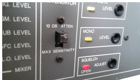
Figure 6: After realignment, signal levels well below -78.2 dBm resulted in squelch opening and test tone detection.
