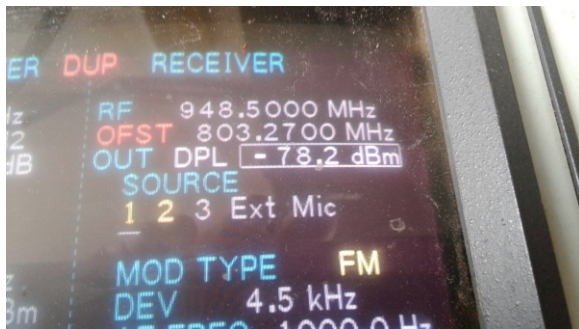
Figures 4 and 5: With front-end of receiver realigned, a -78.2 dBm signal would produce a "0" level on the Marti receiver with the receiver's 10 dB attenuation switch turned on.
